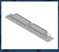
Machine platform with stairs, spiral stairway and ladder. Here as well, the support posts are placed only on the exterior edges of the footprint to utilise the space efficiently.
